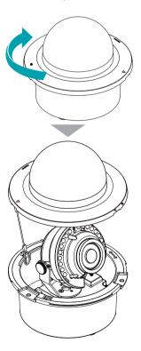
2 Turn the camera body counterclockwise while pressing the body hook of the bottom cover to remove the camera body from the bottom cover.
