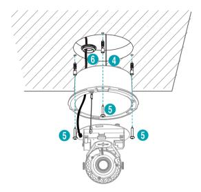
7 Connect the camera body to the bottom cover. Match the cable access hole position of bottom cover and camera body as the following image and turn the camera body clockwise to fix it. Connect the safety wire provided with the camera to the bottom cover and camera body to prevent the camera body from falling.
