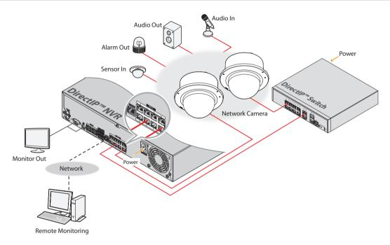
DirectlP $^{\text{IM}}$  NVR makes it easy to use cameras without extra network configurations. Each camera can be controlled via the DirectlP $^{\text{IM}}$  NVR setup menu, without any PC. For detailed camera settings, please see the camera setting pages of DirectlP $^{\text{IM}}$  NVR manual.
