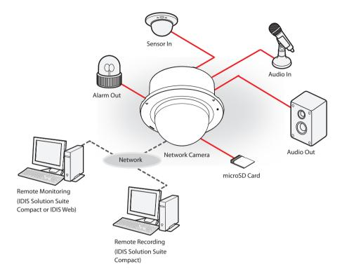
Control the camera over the network from software installed on a computer. Ideal for using the camera over the network from a remote location.
